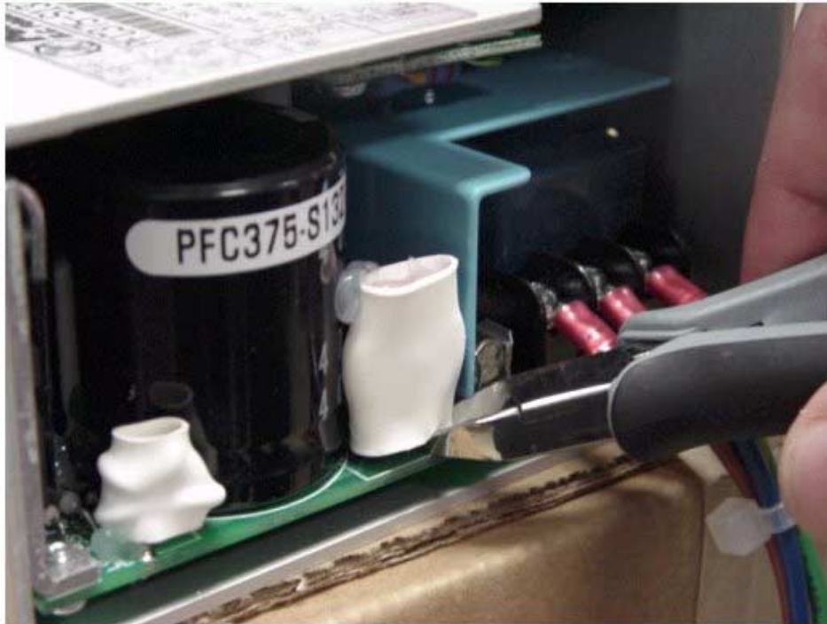
Figure 7. MOV shown while being removed by use of wire cutting pliers.
